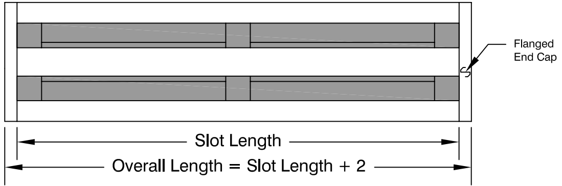
DRYWALL OPENING FOR FLUSH FLANGE AIR BAR WITH FLANGED END CAPS
